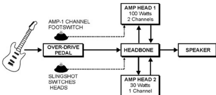
Why is this setup so cool? Because it truly covers all of the bases: the powerful clean sound from a 100-Watt amp is radically different than a cranked all-tube 30-Watt amp. A Headbone setup lets you quickly access the tones from two amps with the convenience of footswitch control right on your pedalboard. Best of all, you only have to carry around a single speaker cabinet - a luxury that is best appreciated at two in the morning after the gig!
