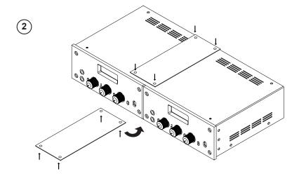
Use 8 small screws to secure the HDI's to each other with the large rectangular braces on the top and bottom of the units.
