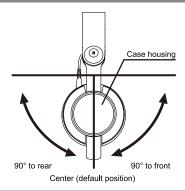
These headphones are designed to allow sound monitoring with one ear by rotating the opposite earphone housing (left or right) up and away from the ear. To rotate the earphone on one side, hold the housing case and rotate it forward or back 90° away from the ear.
