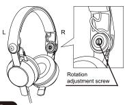
The rotation resistance (tightness) can be adjusted by loosening or tightening the rotation adjustment screw as shown in the illustration.
