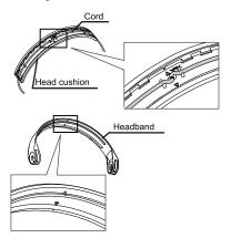
8. Insert the L-R cable divider into the groove at the bottom of the L-side unit, and press the cable along the groove. When pressing the L-R cable divider into the groove, the process will be easier by following the direction indicated in the illustration, and ending by aligning the screw holes.
