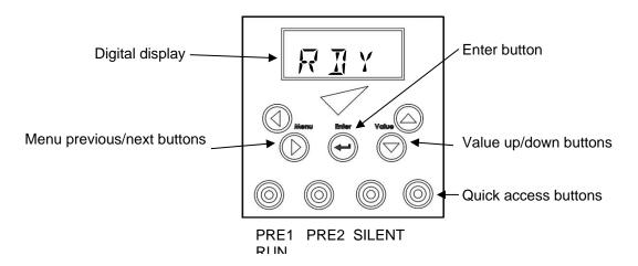
The brightness of the display can be changed to LOW, NORM or HIGH using the DISP menu option.
