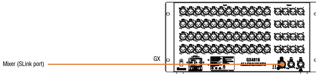
Switch on the mixer first, then the GX Expander. The GX port Lnk/Err indicators flash at a steady rate when the link is established. The red error indicator lights if a communication error is detected.
