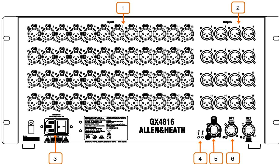
**1 Input sockets** – Balanced XLR mic/line inputs with +48V Phantom Power indicator. The preamps are built into the GX4816 and their Gain, Pad and +48V are controlled from the mixer via the Cat5 link.
