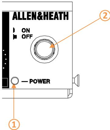
**1 POWER INDICATOR** – LED indicator showing the unit has power. Also used to indicate when unit is in 'Programming' mode (see section 6.4).
