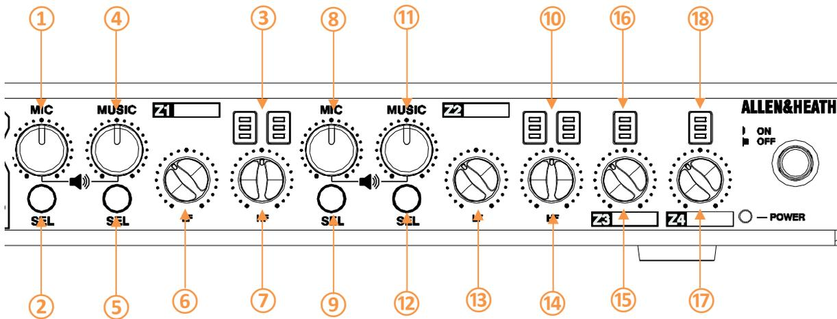
**① Z1 MIC MIX OUTPUT LEVEL** – Adjustable rotary level control for MIC Mix to Zone 1. Output level control Off to +6dB.
