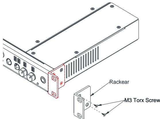
**Be sure to use the supplied screws or exact replacements (damage to internal PCB's can result when using longer screws).**
