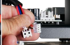
5. Locate the 2-pin and 4-pin Control Module connectors and carefully unplug them from their connector bases. DO NOT USE FORCE TO REMOVE CONNECTORS!
