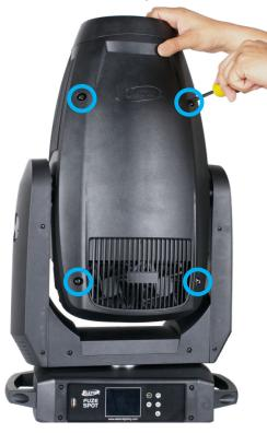
2. Unfasten and remove the front back panels; each and with secured (4x)14-turn Phillips-head screws. (These screws are integrally installed in both panels and cannot be removed.) With the panel screws unfastened, unclip their safety cables to remove them completely from the fixture.
