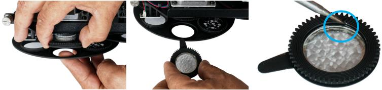
10. REPLACING A ROTATING GOBO Locate the specific Rotating GOBO to replace. Carefully grip the GOBO Holder using your index finger and gently lift it slightly, and then with your fingers pull it out and away until it fully clears the GOBO Wheel. Now locate the tab of the spring, and with a precision pick (or similar tool), carefully press retaining spring inward to relieve tension.
