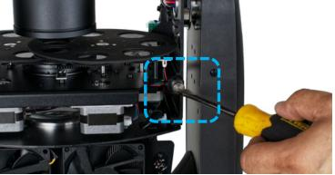
8. Loosen the (2x) slotted thumb screws that secure the GOBO Wheel Module.
