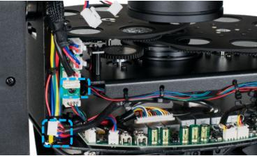
7. Locate the 4-pin GOBO Wheel Module connector and carefully unplug it from the connector base. DO NOT USE FORCE TO REMOVE CONNECTOR!
