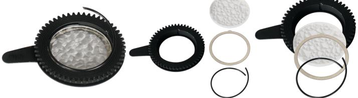
11. Remove the retaining spring and carefully separate the GOBO from the GOBO Holder. Install the replacement Rotating GOBO following the steps above in reverse order.
