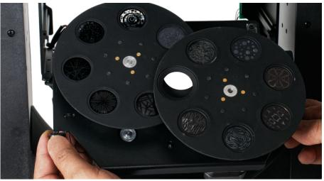
**9.** Carefully grip the GOBO Wheel module and slide it out and away to clear the mounting rails, and then carefully place the module on a stable flat surface in an **INDOOR DUST FREE** location.
