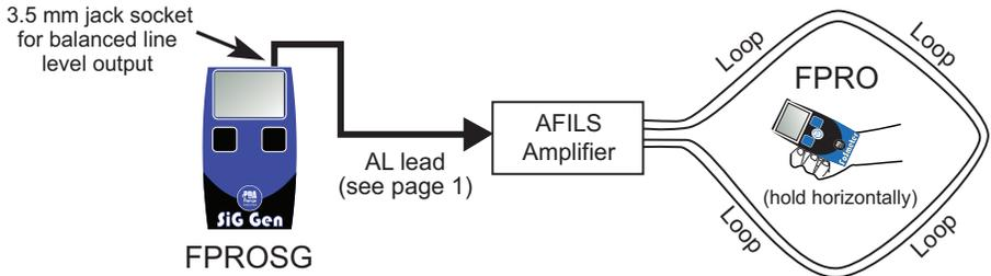
2. Switch on the amplifier and adjust the input signal control and loop drive current in accordance with the amplifier's manual.
