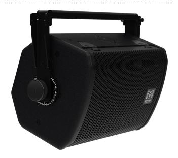
Its exemplary dispersion pattern is achieved by incorporating a dedicated waveguide within the magnet structure which merges into a specially shaped, asymmetric LF cone. With the waveguide and cone combining to form the HF horn, this innovative arrangement avoids a separate 'add-on' horn which would impede the wavefront from the cone and cause irregularities in the frequency response. It also improves on conventional through-the-pole coaxial designs, which can suffer from high frequency beaming.
