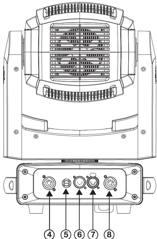
**DMX-512:** DMX is short for Digital Multiplex. This is a universal protocol used as a form of communication between intelligent fixtures and controllers. A DMX controller sends DMX data instructions from the controller to the fixture. DMX data is sent as serial data that travels from fixture to fixture via the DATA “IN” and DATA “OUT” XLR terminals located on all DMX fixtures (most controllers only have a DATA “OUT” terminal).
