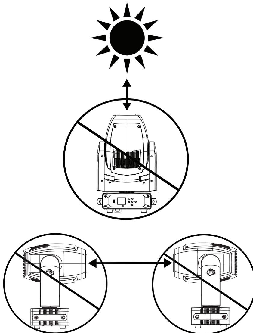
**NOTICE:** The suitable environmental temperature for this lighting fixture is between -25° C to 45° C. Do not place this lighting fixture in an environment where the temperatures are under or above the temperatures stated above. This will allow the fixture to run at its best and help prolong the fixture life.
