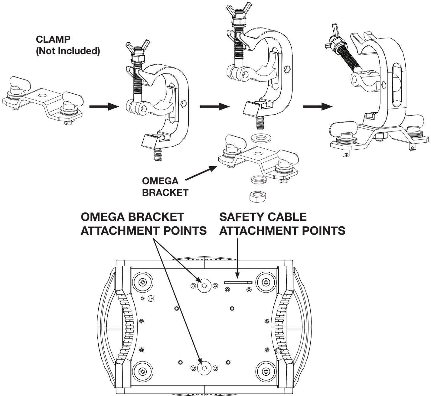
Screw one clamp via a M12 screw and nut into the Omega bracket. Insert the quick-lock fasteners of the Omega bracket into the respective holes on the bottom of the Focus Spot 5Z. Tighten the quick-lock fasteners fully clockwise. Pull the safety cable through the opening located on the base plate and over the trussing system or a safe fixation spot. Insert the end in the carabine and tighten the safety screw.
