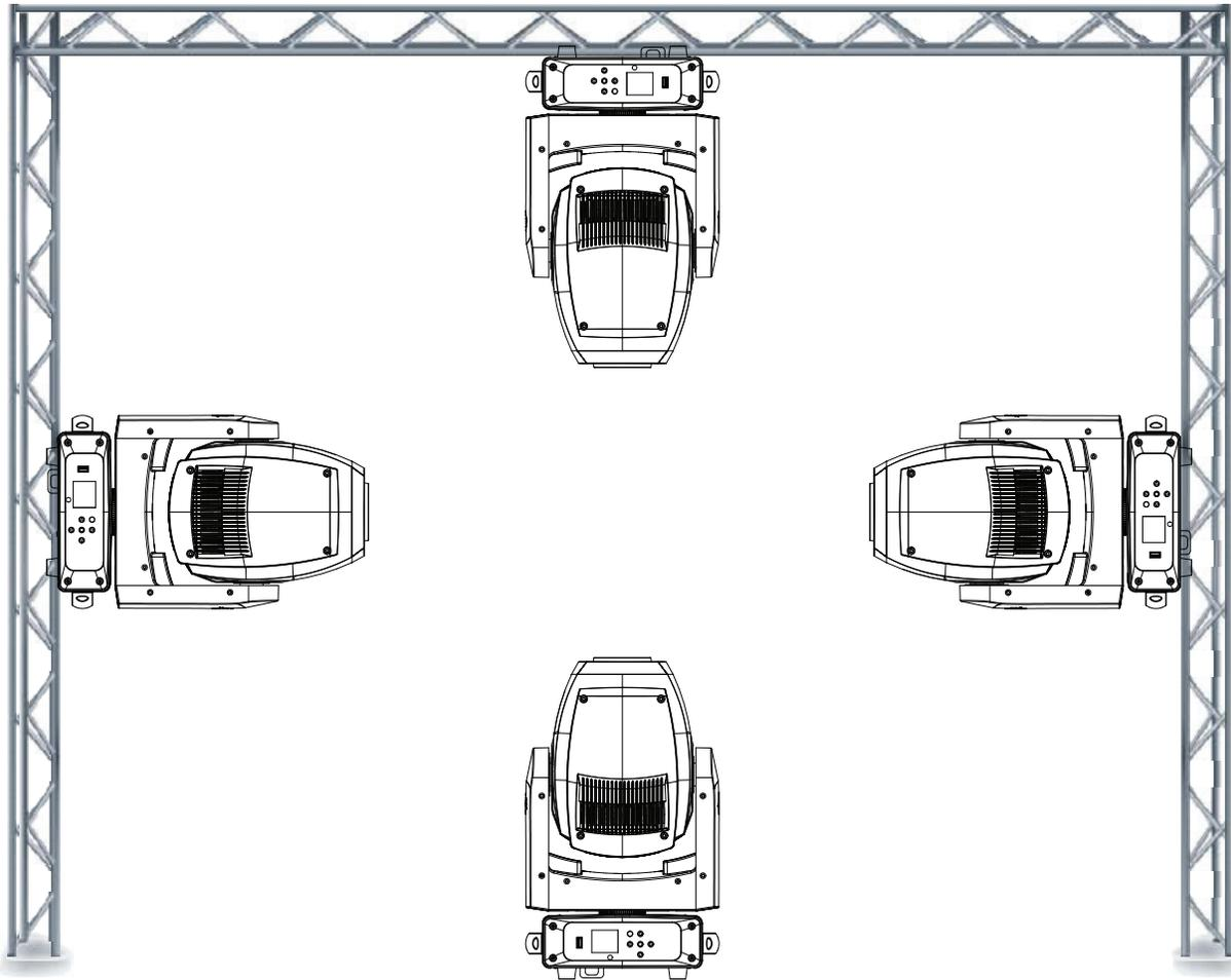
The Focus Spot 5Z is fully operational in three different mounting positions, hanging upside-down from a ceiling or trussing, sideways on trussing, or set on a flat level surface. Be sure this fixture is kept at least 12m (40ft) away from any flammable materials (decoration etc.). Always use and install a safety cable as a safety measure to prevent accidental damage and/or injury in the event the clamp fails (see previous page). Never use the carrying handles for secondary attachment.
