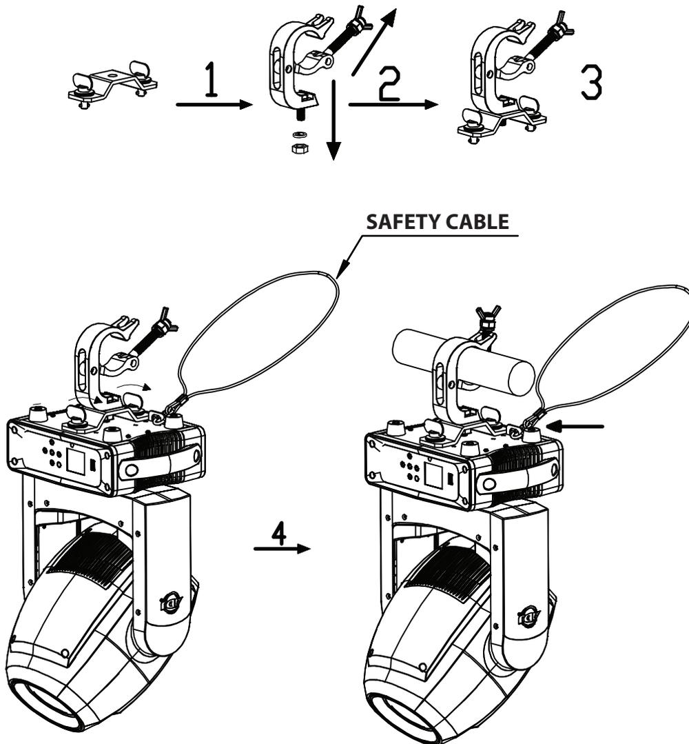
Screw one clamp each via a M12 screw and nut into the Omega bracket. Insert the quick-lock fasteners of the Omega holder's into the respective holes on the bottom of the Focus Spot 4Z/Focus Spot 4Z Pearl. Tighten the quick-lock fasteners fully clockwise. Pull the safety cable through the openings located on the base plate and over the trussing system or a safe fixation spot. Insert the end in the carabine and tighten the safety screw.
