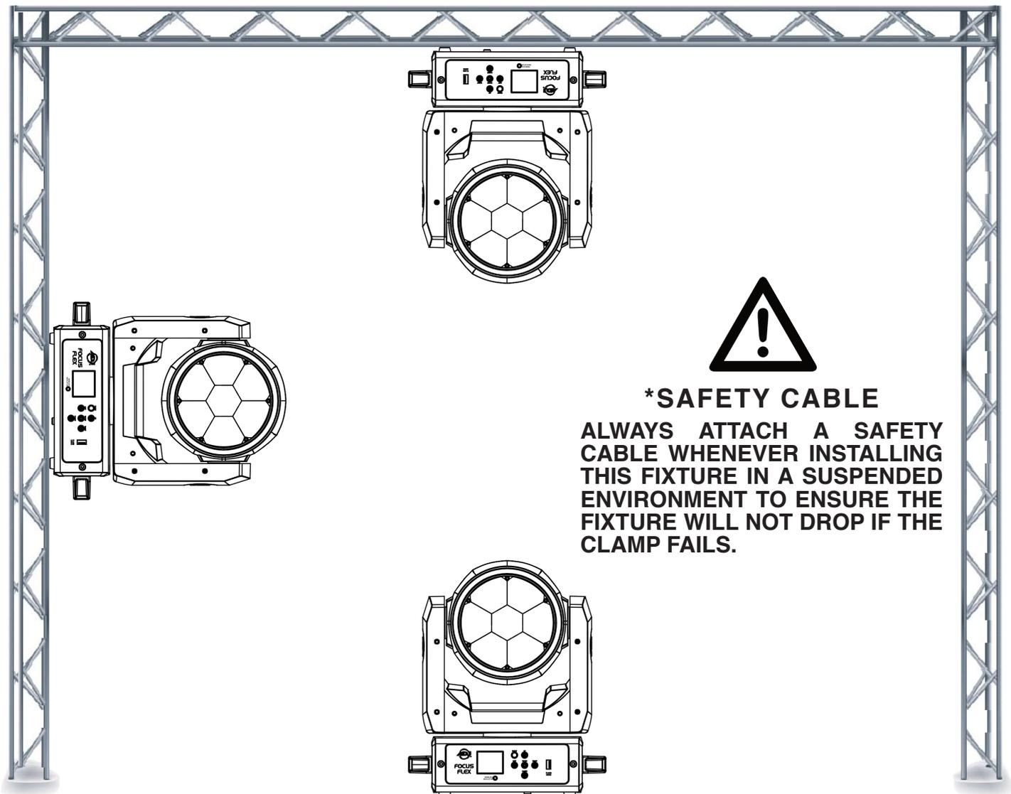
The Focus Flex is fully operational in three different mounting positions, hanging upside-down, mounted sideways on trussing, or set on a flat level surface. Be sure this fixture is kept at least 0.2m (7.9in.) away from any flammable materials (decoration etc.). Always use and install the supplied safety cable as a safety measure to prevent accidental damage and/or injury in the event the clamp fails (see next page). Never use the carrying handles for secondary attachment.
