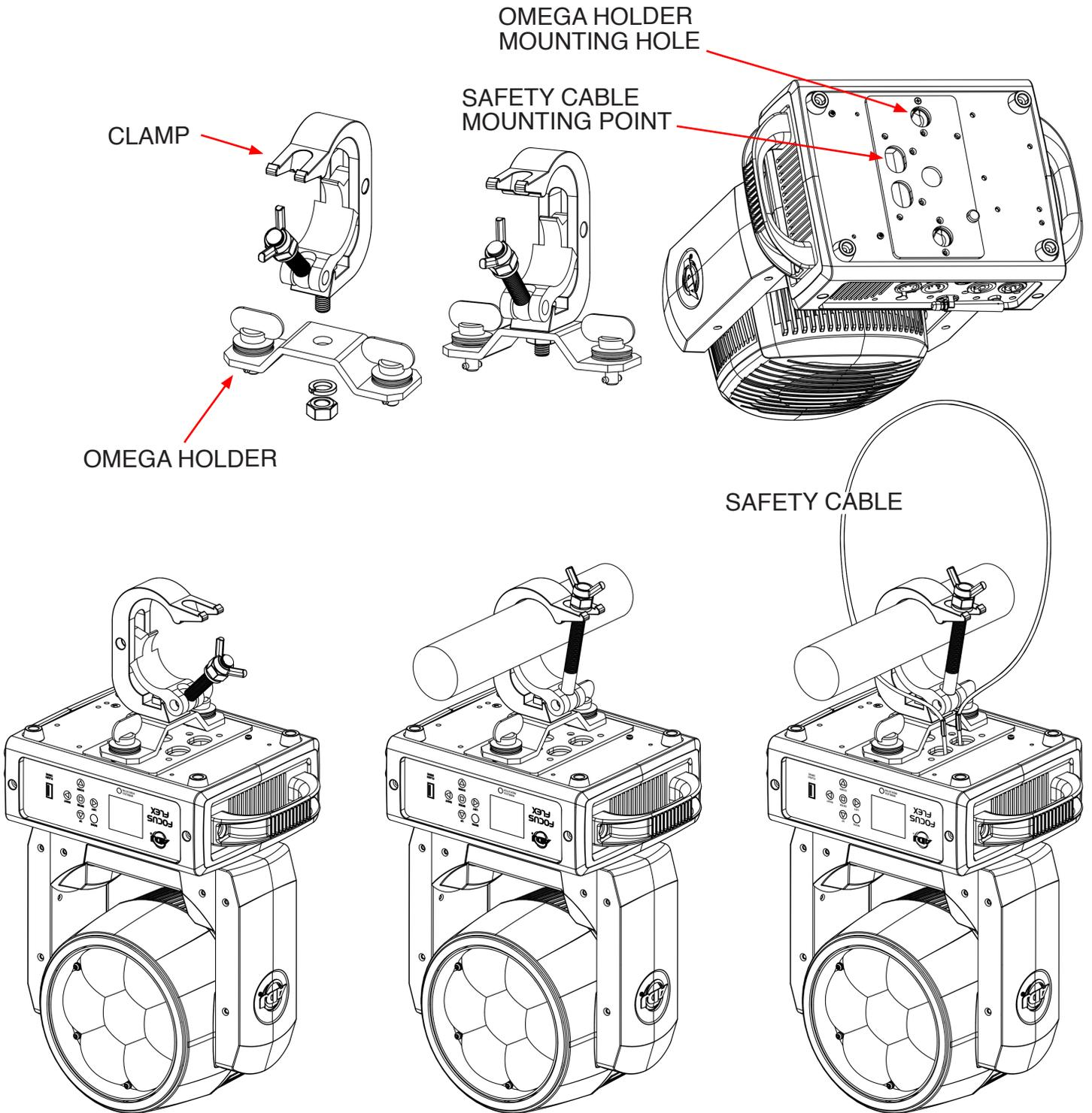
Screw one clamp via a M12 screw and nut into the Omega holder. Insert the quick-lock fasteners of the Omega holder into the respective holes of the adjustable mounting bracket. Tighten the quick-lock fasteners fully clockwise. Pull the safety-cable through the opening located on the bottom of the unit and over the trussing system or a safe fixation spot. Insert the end in the carabiner and tighten the safety screw.
