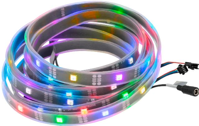
The FLEX PIXEL P40WP™ is an outdoor IP65 rated 10 foot (3m) flexible LED pixel tape featuring (72) RGB SMD tri-color LED pixels (216 total DMX channels) spaced on 1.6" (40mm) centers, producing over 1 billion color possibilities with a 120° viewing angle, enclosed in an IP65 rated waterproof flexible cover which can be cut and extended every 4" (102mm), and mountable to most surfaces using Elation's FLEX CHANNEL™ line of aluminum mounting tracks.
