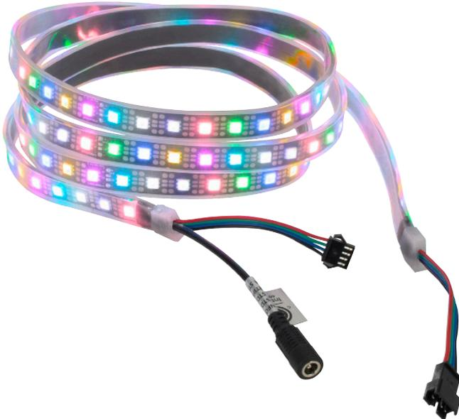
The FLEX PIXEL P14WP™ is an outdoor IP65 rated 6.6 foot (2m) flexible LED pixel tape featuring (144) RGB SMD tri-color LED pixels (432 total DMX channels) spaced on 0.55" (14mm) centers, producing over 1 billion color possibilities with a 120° viewing angle, enclosed in an IP65 rated waterproof flexible cover which can be cut and extended every 2" (51mm), and mountable to most surfaces using Elation's FLEX CHANNEL™ line of aluminum mounting tracks.
