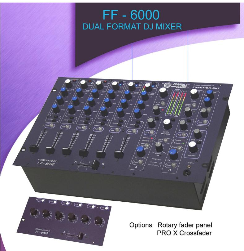
The features and layout of the FF-6000 were determined in collaboration with Funktion One and leading DJs world wide. The result is a mixer which is of the highest sound quality (frequency response 20Hz - 20Khz +/- 0.5db, THD + Noise @ 1Khz <0.01%).
