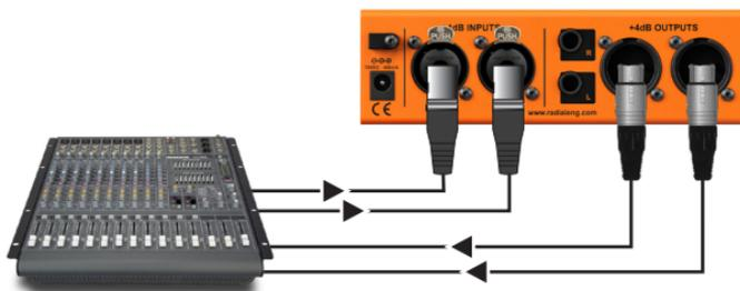
*Connecting a mixer to the EXTC Stereo using XLR cables*
