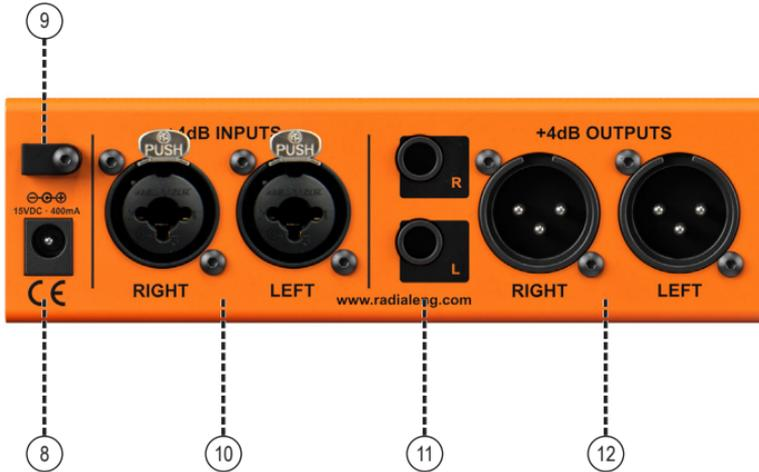
9. **CABLE CLAMP:** Affixes the PSU cable to the EXTC Stereo to prevent accidental disconnection.
