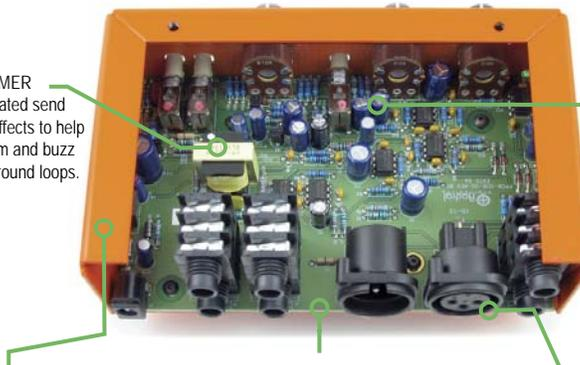
I-BEAM REINFORCED - Enclosure makes it impossible to torque the PC board & eliminates cold solder joints.
