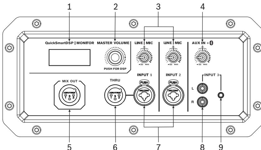
1. **LCD** – DSP control and monitoring interface.
