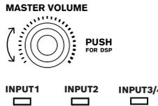
7. Using the **MASTER VOL knob**, adjust the volume (**VOL**) until you get the required output from the loudspeaker.
