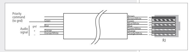
Important: It is necessary to use the RJ 45 port priority command to open the audio input 2. (for instance, through the BM 3001 paging microphone push-button).
