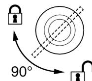
4. Fasten the omega brackets to mounting holes **A** on the base of the fixture using the bracket's quarter-turn fasteners. Turn quarter-turn fasteners a full 90° to lock them (see illustration on right).
