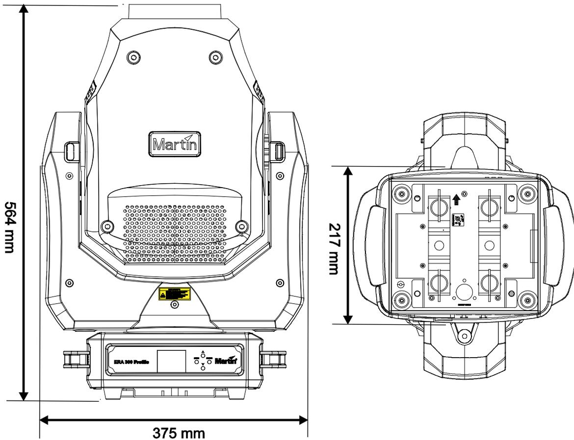
All dimensions are given in millimeters
