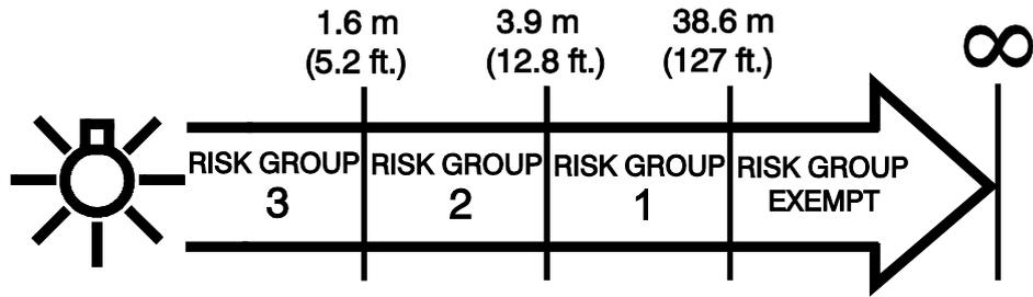
The luminaire should be positioned so that prolonged staring into the luminaire at a distance closer than 3.9 m is not expected.
