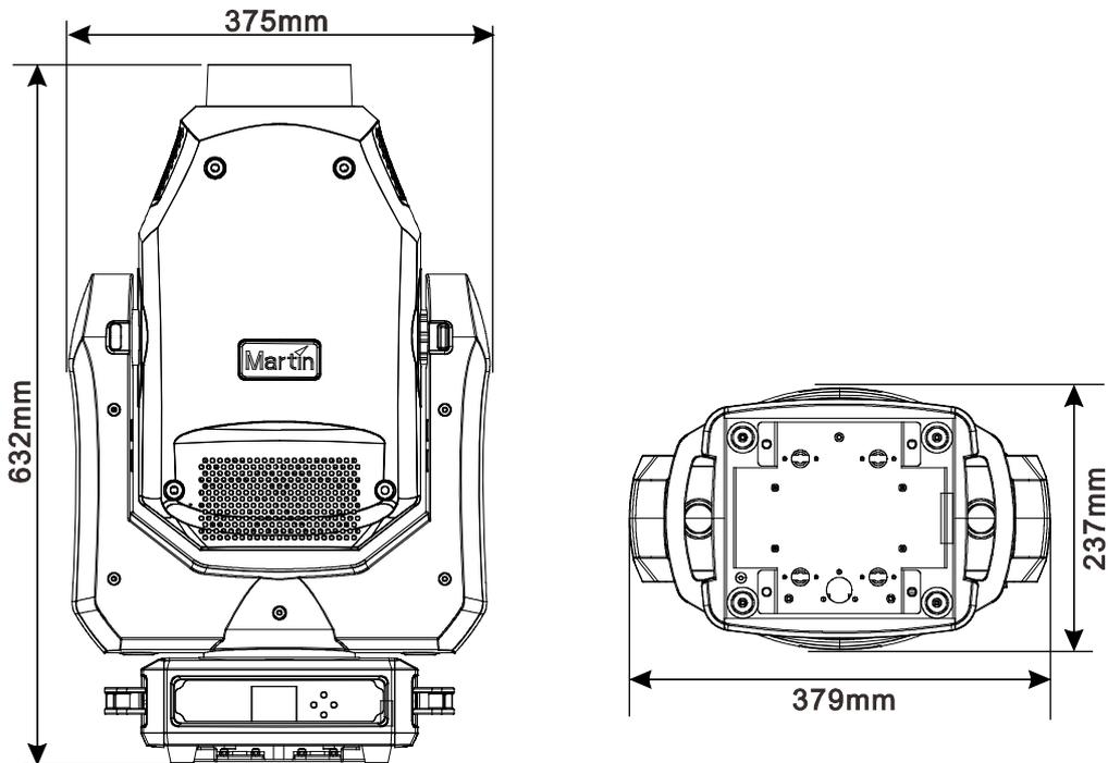
All dimensions are given in millimeters
