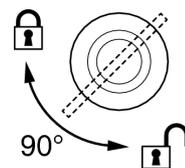
4. Fasten the omega brackets to mounting holes **A** on the base of the fixture using the bracket's quarter-turn fasteners. Turn quarter-turn fasteners a full 90° to lock them (see illustration on right).
