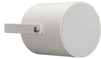
The Apart EN-MP5T20-W is a compact and stylish sound projector made of powder coated aluminium (RAL 9010 equivalent), equipped with a high efficiency full range driver and a multi tap 100 volt transformer, all certified according EN 54-24. The unit is equipped with a ceramic speaker line connector block, junction box, thermal fuse and stainless installation bracket.
