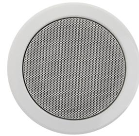
The Apart EN-CMX6T10 is a built-in 2-way ceiling speaker made of powder coated steel (RAL 9010 equivalent), equipped with a high class 2-way speaker and a multi tap 100 volt transformer, all certified according EN 54-24, offering a detailed and powerful sound for demanding applications.
