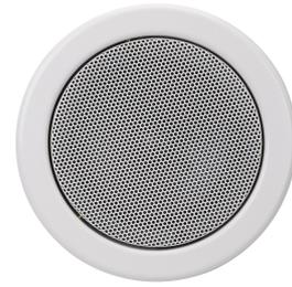
The Apart EN-CM5T6 is a 5.25" built-in ceiling speaker made of powder coated steel (RAL 9010 equivalent), equipped with a high efficiency full range speaker and a multi tap 100 volt transformer, all certified according EN 54-24.
