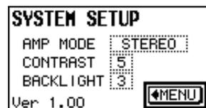
2. Turn the [MENU/CONTROL] rotary encoder until the cursor highlights the AMP MODE parameter box.
