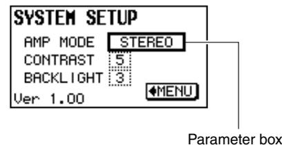
3. Press the [MENU/CONTROL] rotary encoder so that the parameter box is fully highlighted.
