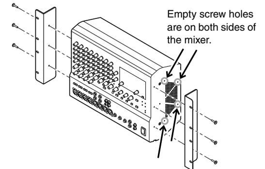
4. If you wish to remove the rack-mount brackets and reinstall the side pads, ensure that they are installed on the correct sides of the mixer. The inside surface of the side pads are marked as "L" (Left) or "R" (Right).
