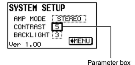
3. Press the [MENU/CONTROL] rotary encoder so that the parameter box is fully highlighted.
