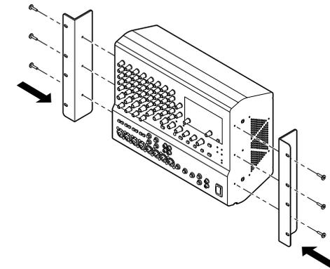
3. Carefully store the remaining six screws that are not used in Step 2 so they are not lost. Once the rack-mount brackets are installed there will be a total of eight empty screw holes on the both sides of the mixer.
