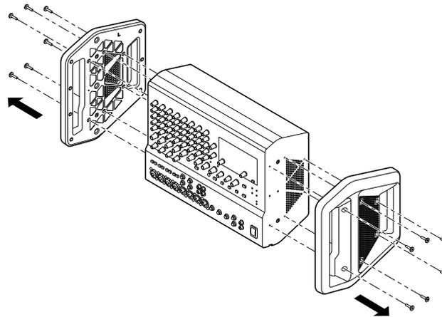
2. Use six of the screws you removed in Step 1 to securely install the RK-EMX7 separately sold (rack-mount brackets) onto the mixer.
