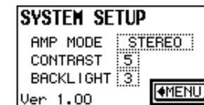
2. Turn the [MENU/CONTROL] rotary encoder until the cursor highlights the CONTRAST parameter box.
