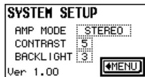
2. Turn the [MENU/CONTROL] rotary encoder until the cursor highlights the BACKLIGHT parameter box.
