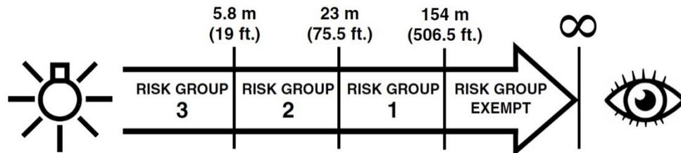
At a distance of less than 5.8 m (19 ft.) from the fixture, the light output can potentially cause eye or skin injury before an exposed person's natural aversion responses (blink reflex and reaction to skin discomfort) can protect them. At distances greater than 5.8 m (19 ft.), potential eye and skin injury hazards from the light output are normally prevented by natural aversion reflexes.
