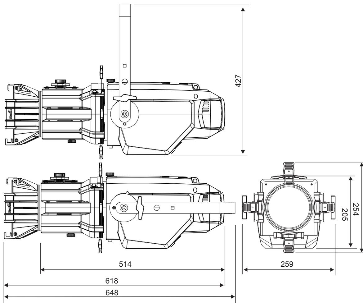
All dimensions are given in millimeters.
