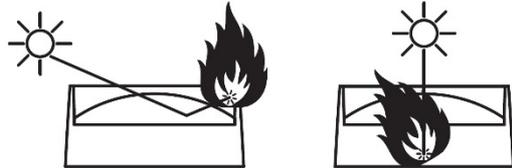
**Important!** Do not point the output from other lighting fixtures at the fixture, as powerful light can damage the display.
