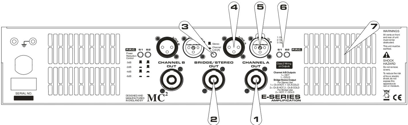
1: Channel A output Speakon socket: Output is wired pins 1+: hot, 1-: cold. Similarly channel B's output Speakon socket uses two poles wired as above.
