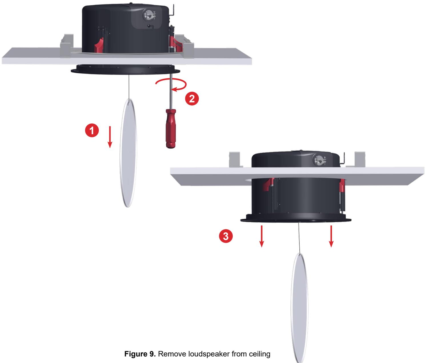
Figure 9. Remove loudspeaker from ceiling
