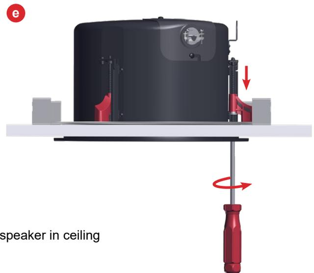
**Figure 5.** Install and secure loudspeaker in ceiling
