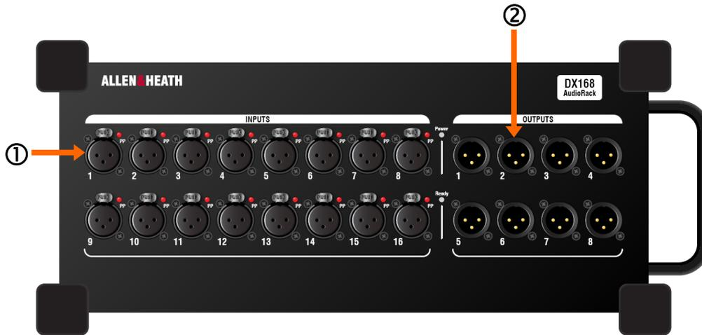
① **Input sockets** 16 balanced XLR mic/line inputs with +48V Phantom Power indicator.
