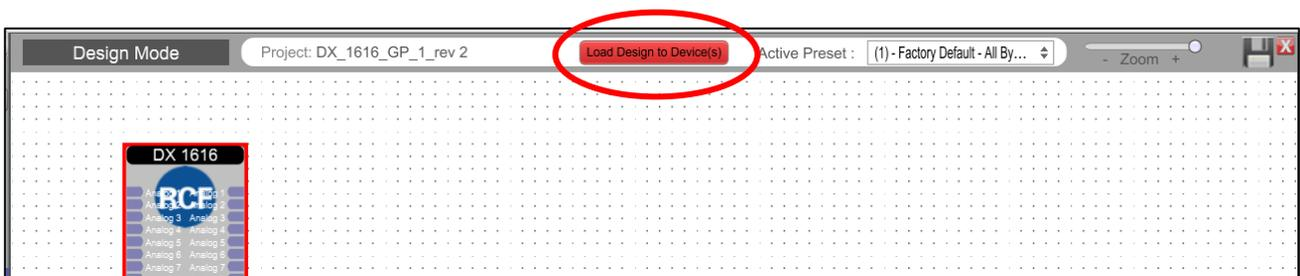
Figure 15: Load Design to Devices
