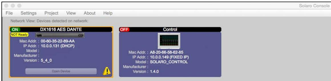
Figure 9: Firmware update – device not ready is shown
