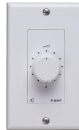
The Apart D-VOL60 is a 70 volt volume control. It can handle up to 60 watts of power and is very durable thanks to the step-by-step attenuation in 11 steps + zero position. The D-VOL60 is designed to handle 24V priority signals. This means that you can always get an announcement out, even to zones where the local volume control is in the 'OFF' position! If your amplifier has a 24V priority output, it will send a 24V signal when you push the talk button on the microphone.
