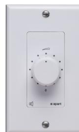
The Apart D-VOL120 is a 70 volt volume control. It can handle up to 120 watts of power and is very durable thanks to the step-by-step attenuation in 11 steps + zero position. The D-VOL120 is designed to handle 24V priority signals. This means that you can always get an announcement out, even to zones where the local volume control is in the 'OFF' position! If your amplifier has a 24V priority output, it will send a 24V signal when you push the talk button on the microphone.
