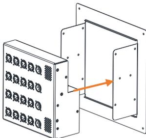
**Flush mounting in a wall** Use the mounting frame AH11504 in the orientation shown below. Align the threaded inserts on the sides of the DT164-W with the frame, and secure the unit in place with the 6x M4 6mm T20 screws provided. Connect the power and Cat5 cable/s, then fix the assembly to the wall using appropriate fixings or screws for the type of wall.
