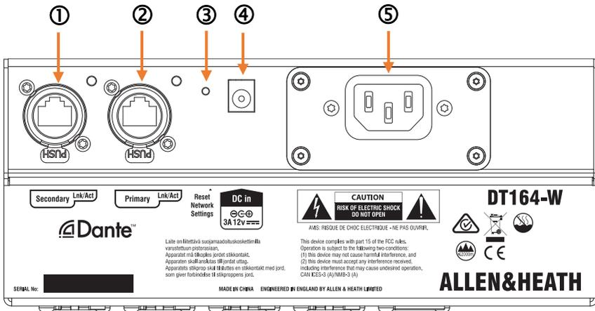
① **Dante Secondary** Can be set to Redundant mode or to Switched mode for connection to multiple devices, for example two mixing consoles. Set the port mode in Dante Controller.
