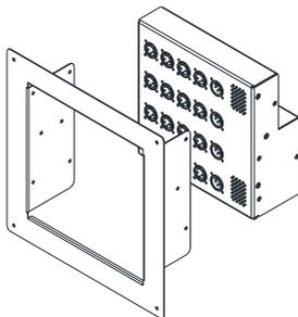
**Floor mounting** The DT164-W can be mounted in a floor box / stage pocket / dip trap. It must be installed in accordance with local installation and wiring regulations. We recommend using the **ACE Backstage 174SLBK** stage pocket system for use with the DT164-W.
