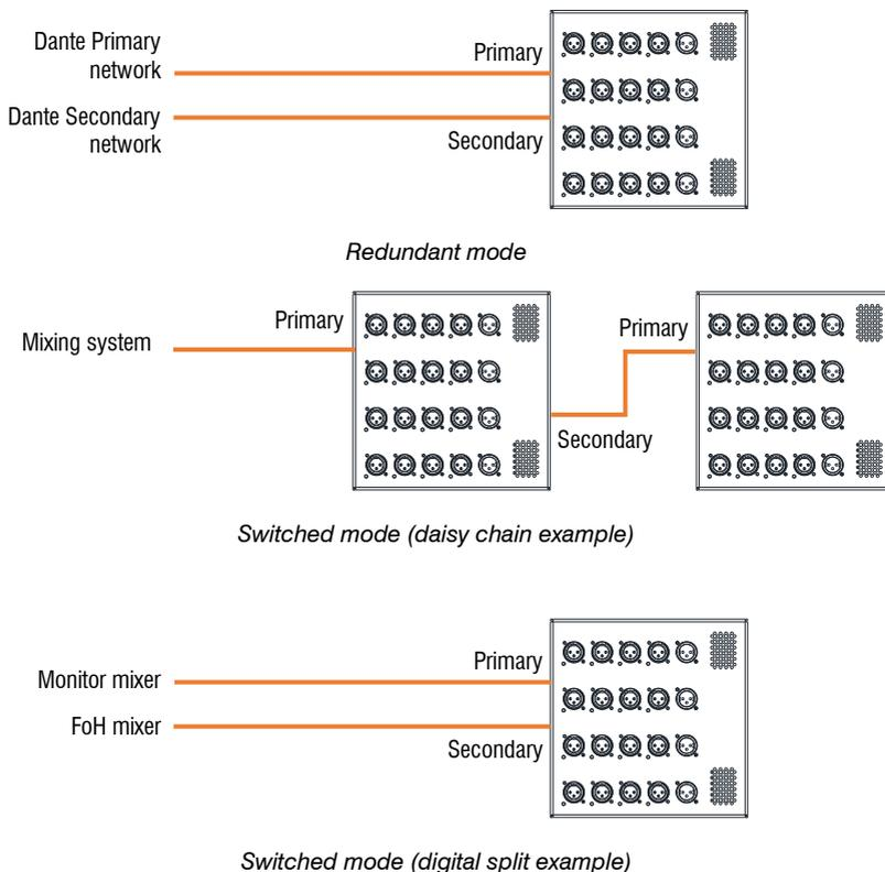
ⓘ A maximum of 32 DT Expanders (DT168 or DT164-W) can be connected on the same Dante network.
