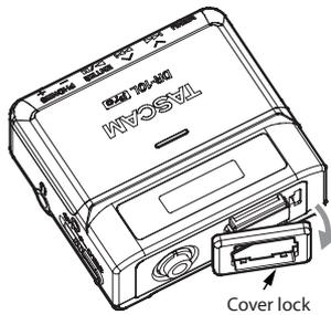
2. After removing the connector cover, insert the AK-BT1 into the unit.
