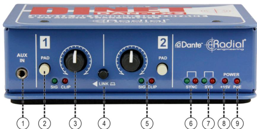
1. **3.5MM INPUT:** Stereo TRS input for use with laptops, tablets and smartphones. Wired in parallel with the XLR and RCA inputs.
