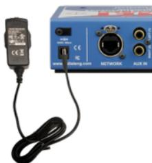
As a backup option, the DAN-TX2 is designed to be able to have both PoE and the 15VDC adaptor connected at the same time. If one fails, the other will maintain power without interruption.
