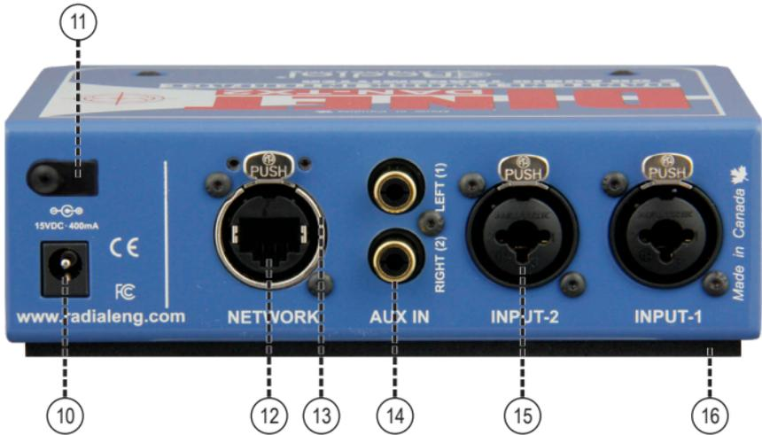
10. **POWER:** 15VDC connection for use with included Radial power adapter when PoE is not available.
