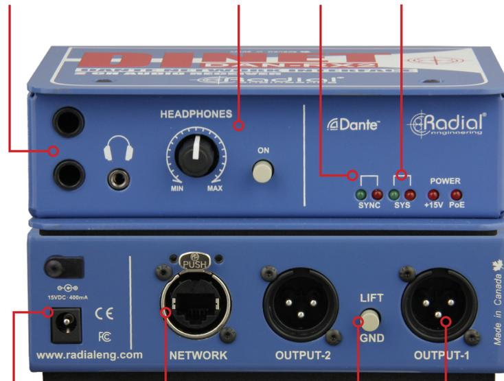
**POWER** - 15VDC connection for use with included Radial power adaptor when PoE is not available.
