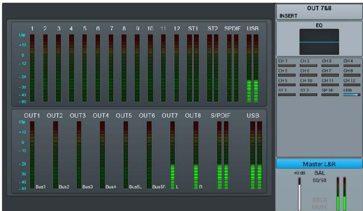
While the left side of the page gives a full overview of all in- and outputs of the console, the right side shows the Master L/R output strip, which in functionality follows exactly the stereo Busses 5-8. The meter settings (pre- / post-fader) can be adjusted on the meter page in Settings, which can be opened by yet another swipe to the right or by pressing the Settings button on the front panel.
