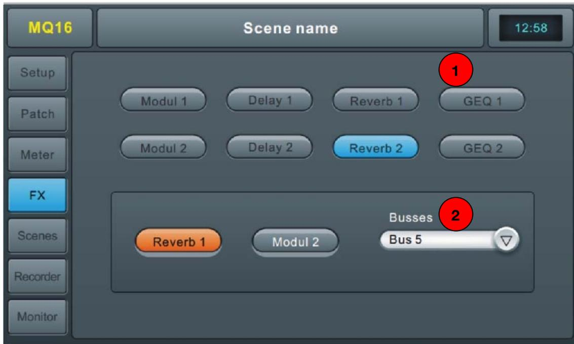
The Effects has 8 modules, which are 2 Modulation, 2 Delay, 2 Reverb and 2 15-band GEQ. Each module can be inserted to an input processing channel or bus processing channel only once. You can insert up to two effects into a bus or channel. For example reverb & delay to create a vocal effect.
