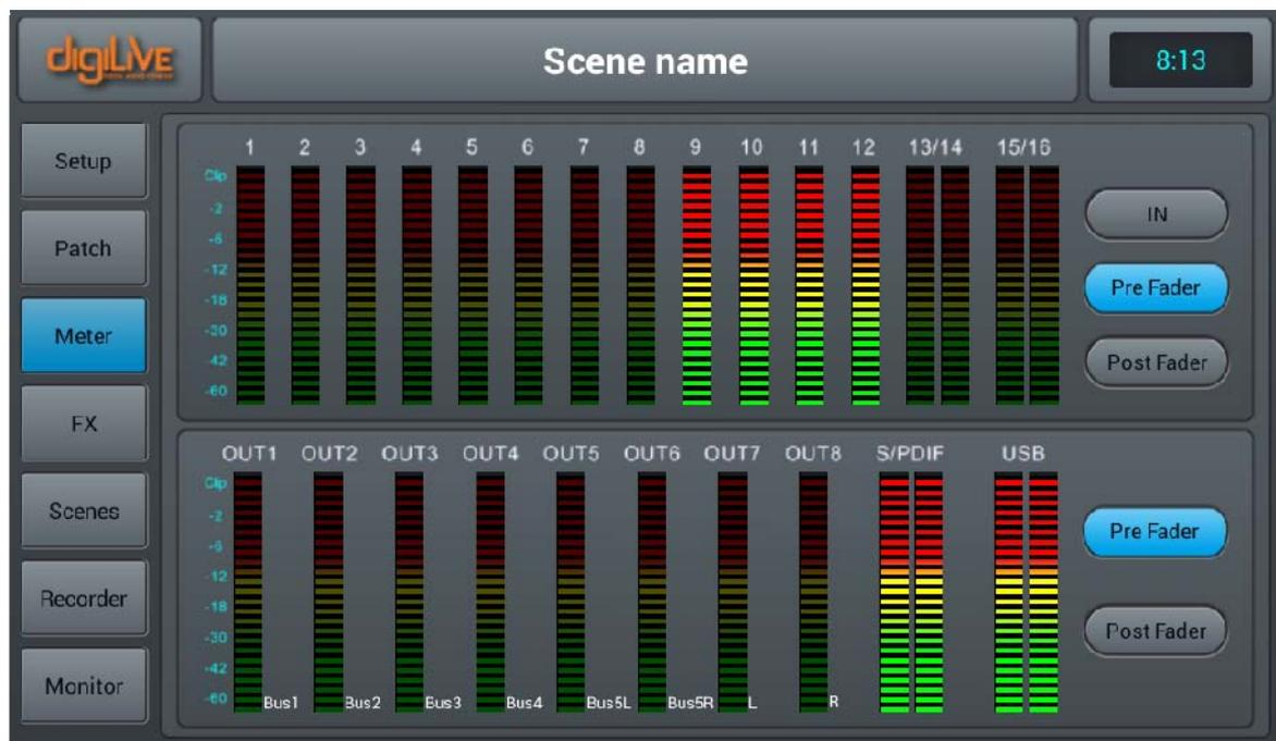
Signal level of input processing channel has three modes—IN, Pre Fader and Post Fader with Pre Fader as the default. Signal level mode displayed can be changed with a button press.
