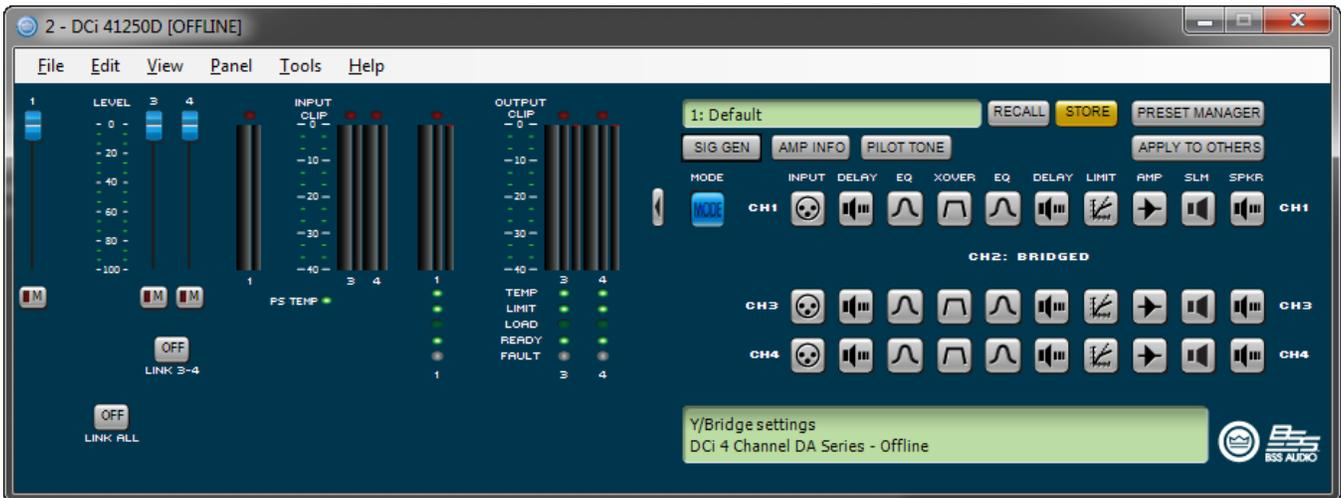
Figure 20: DSP chain configured for bridge mono operation
