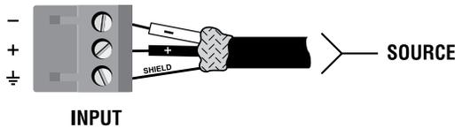
Figure 3: Balanced wiring
