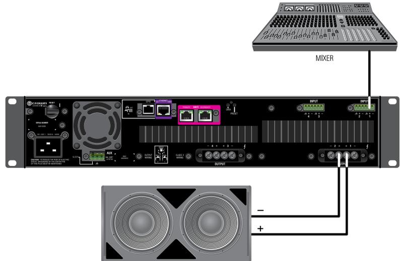
**Figure 23:** System wiring in Bridge Mono mode
