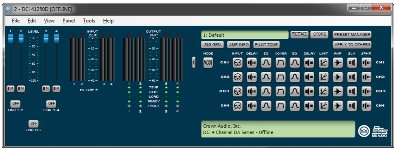
Figure 39: Onboard DSP controllable from Configuration panel
