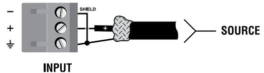
Figure 4: Unbalanced wiring
