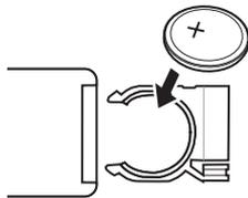
3. Reinsert the battery holder into the remote control.
