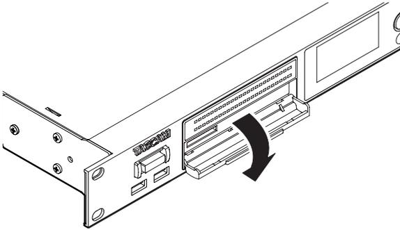
2. Insert the SD card with the correct orientation. The label should be facing up and the contacts facing in.
