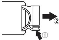
2. Install a coin-shaped lithium ion battery (CR2025) into the holder with the correct  $\oplus/\ominus$  orientation.
