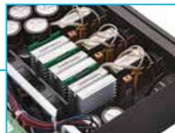
Regulated Switch-Mode Power Supply (R.SMPS)
