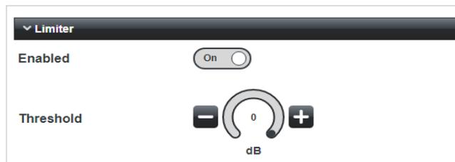
The limiter is active by default; it may be disabled by setting the **Enabled** switch to **Off**.
