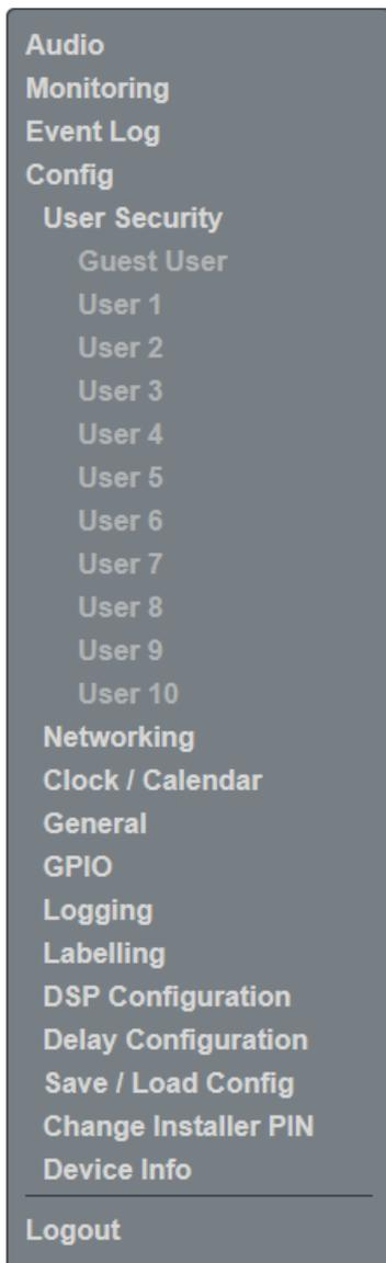
The User security system allows up to ten Users - *in addition to the Installer* - unique PIN access to the control pages. Additionally, a Guest User may access the control pages without a PIN. Clicking on any of **User 1** to **User 10** opens the User privileges page for that User:
