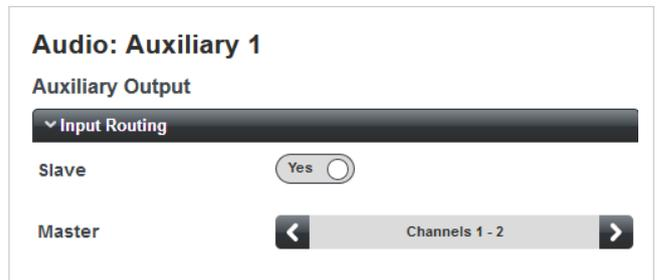
Auxiliary Outputs are by default mono. When one is slaved to a stereo pair of channels, its source becomes a mono sum of the signals in the two channels. Alternative, mono amplifier channels will be available as sources via the **Master** selector as single channels in the normal way. Source selection for Auxiliary Outputs when they are not in Slave mode is unchanged: any Line Input (or **off**) may be selected.
