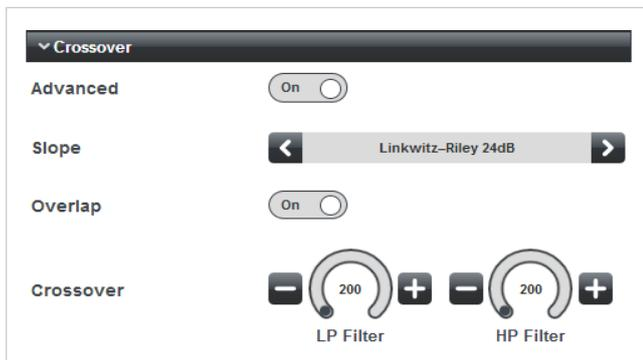
This permits a greater degree of control in tailoring the response of the crossover. Both filter controls have the full audio range of 20 Hz to 20 kHz, and thus the turnover frequencies of each filter section may be adjusted to be as close together or as far apart as wished, the variation determining the flatness of overall frequency response in the crossover region. Again, loudspeaker manufacturers will generally offer recommendations for particular speaker types.
