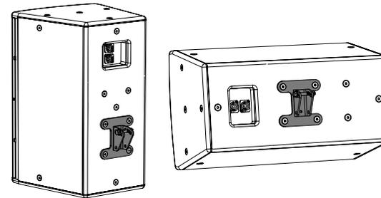
Optional Wall Bracket mounting positions enable greater down-tilt, using the lower four M8 bolt position, or the loudspeaker can be mounted in landscape mode by rotating the bracket as shown:
