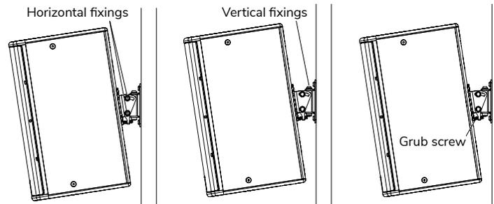
Once the loudspeaker is in position and you are happy with the angle adjustments, tighten all fixings as shown to lock the cabinet in place.
