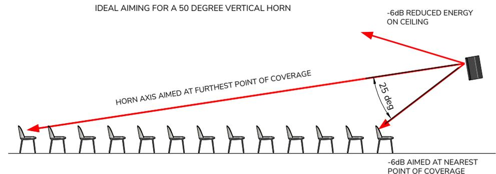
The coverage specifications are useful for informing where the loudspeakers should be aimed. In any horn-loaded loudspeaker, the optimum output is the centre axis of the horn where you have maximum level from the system. It therefore follows that the horn axis should be aimed at the furthest point of the audience.
