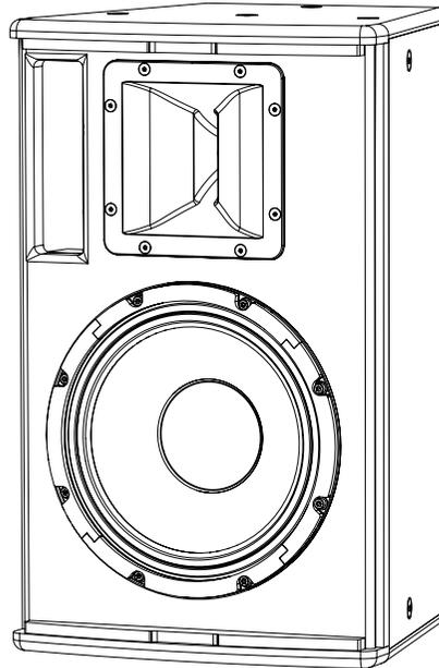
Rotatable high frequency horn, low frequency driver, bass reflex port, M8 fixings
