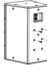
Remove M8 fixing bolts from the rear of the loudspeaker cabinet
