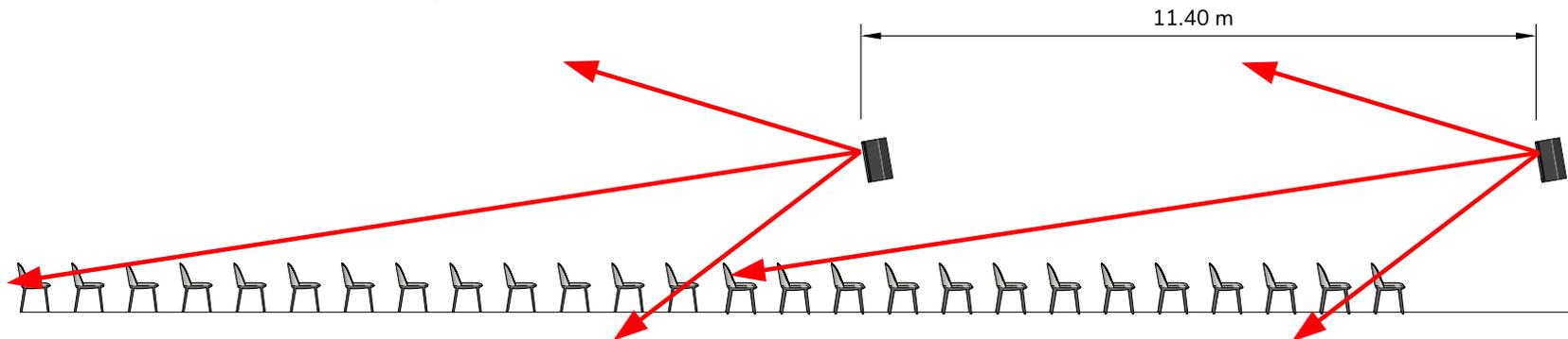
Because of this level drop over distance, in larger rooms it's well worth considering additional loudspeakers to counter this effect, maintaining volume and intelligibility. In this case, it is important that the second row of loudspeakers down the room are delayed to match the arrival of the sound from the first pair of speakers, as shown above.
