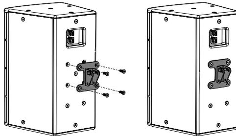
Position loudspeaker cabinet section of Wall Bracket over the four M8 mounting points and secure with the four bolts from the back of the cabinet
