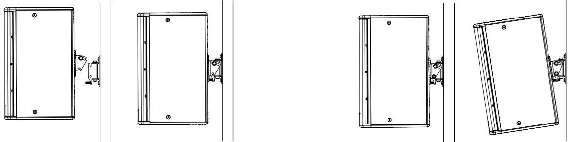
Lift loudspeaker into position making sure that the two halves of Wall Bracket line up – the adjustable bolt sits into the two 'U shaped' cups in the wall section of the bracket
