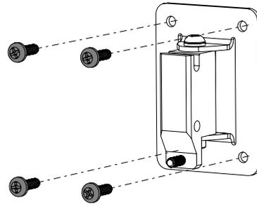
Once loudspeaker position has been decided, affix wall section of Wall Bracket (A,B or C depending on Cuboid model) securely to a suitable wall mounting point
