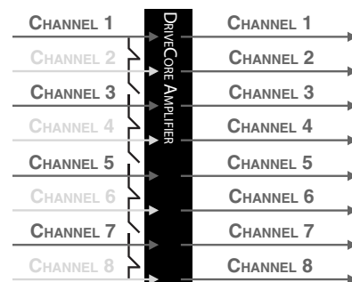
Figure 4.6.5 Four channel to eight channel routing
