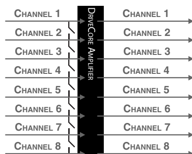
Figure 4.6.2 Eight channels with no input routing
