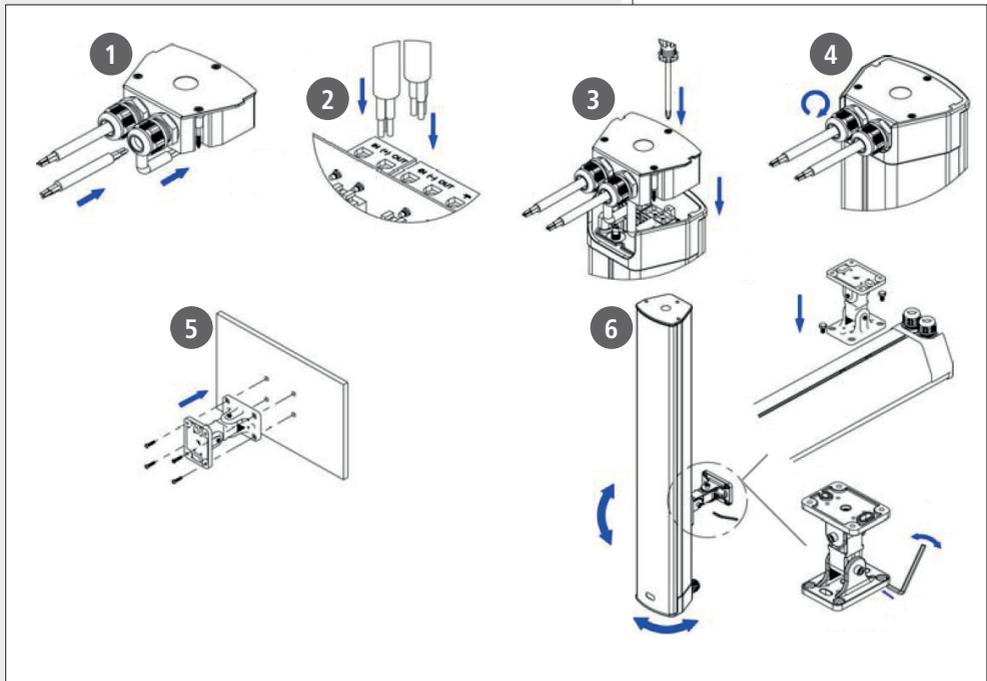
1. Insert cables through the two rear hexagonal cable glands.
