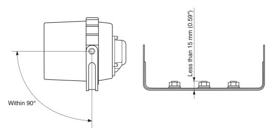
• Do not install the speaker face-up from a horizontal plane nor in such a way that the paper cone is exposed to direct sunlight.
