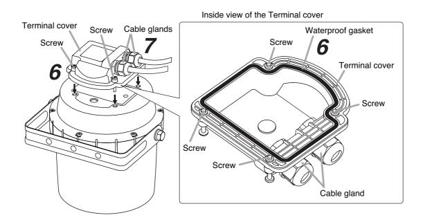
Step 7. Securely tighten the cable glands.
