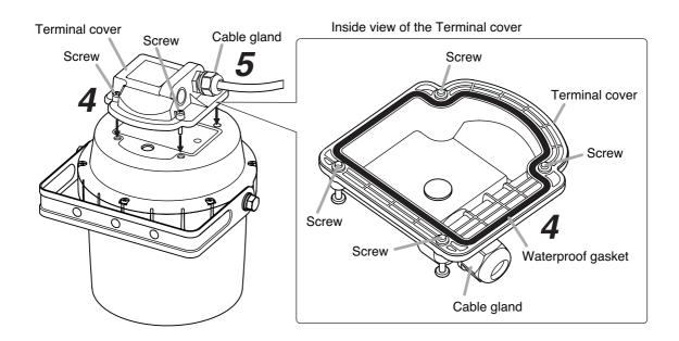
Step 5. Securely tighten the cable gland.
