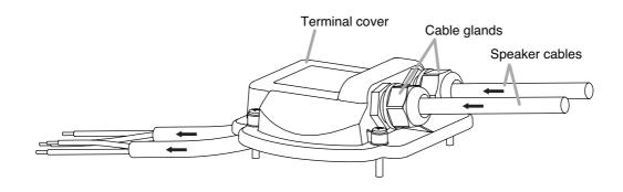
**Step 5.** Connect the speaker cables with the same polarity to each terminal according to the polarity indication at the screw terminal.
