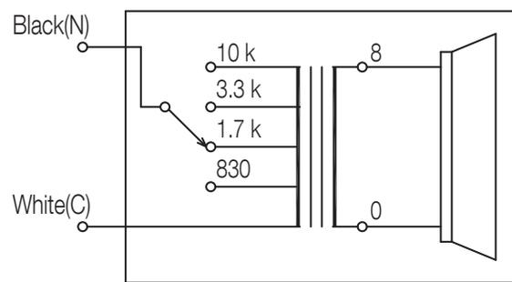
(Transformer connection when the speaker is supplied from the factory)
