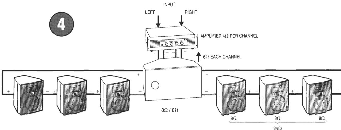
**Series/Parallel** - It is possible to utilize various series/parallel 'hook-up' topologies to increase the number of loudspeakers driven on an amplifier. See diag. 4 for one example of a series/parallel hook-up topology.
