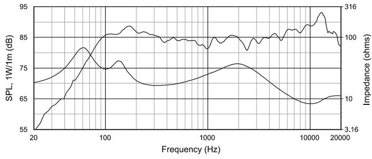
Measured on-axis with a distance referenced to 1 meter at 1 watt.
