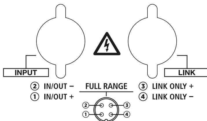
The rear panel displays 2 sockets, both for 'Amphenol eco/mat IP 67' (4-pole) plugs:
