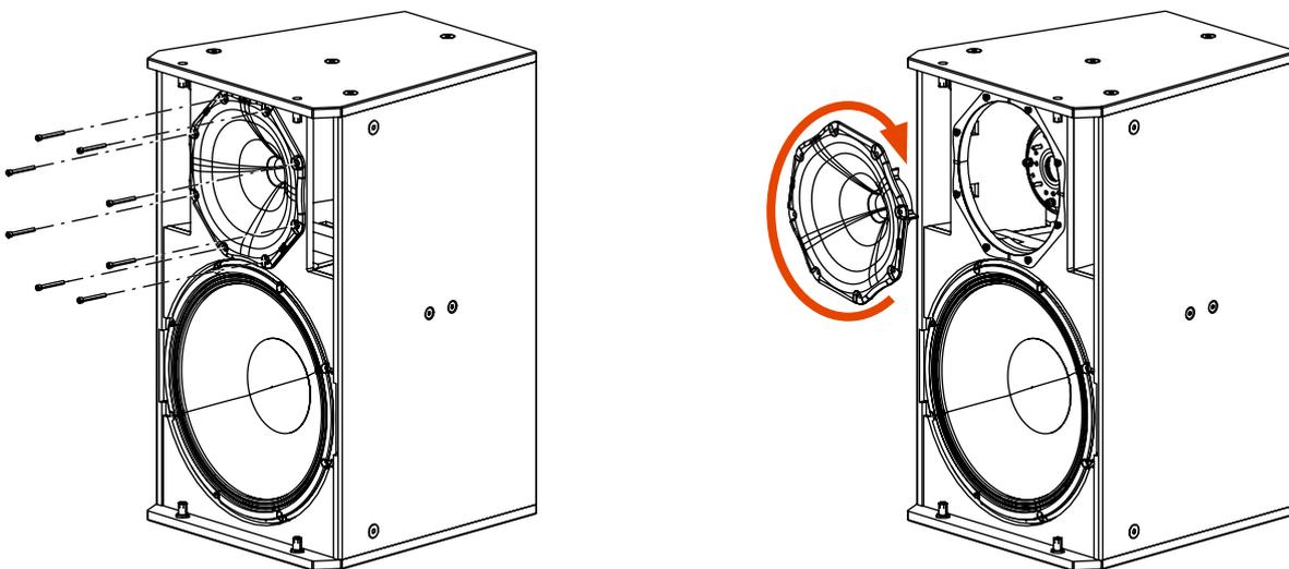
3. Screw back the horn and the grille. The speaker can now be used horizontally.
