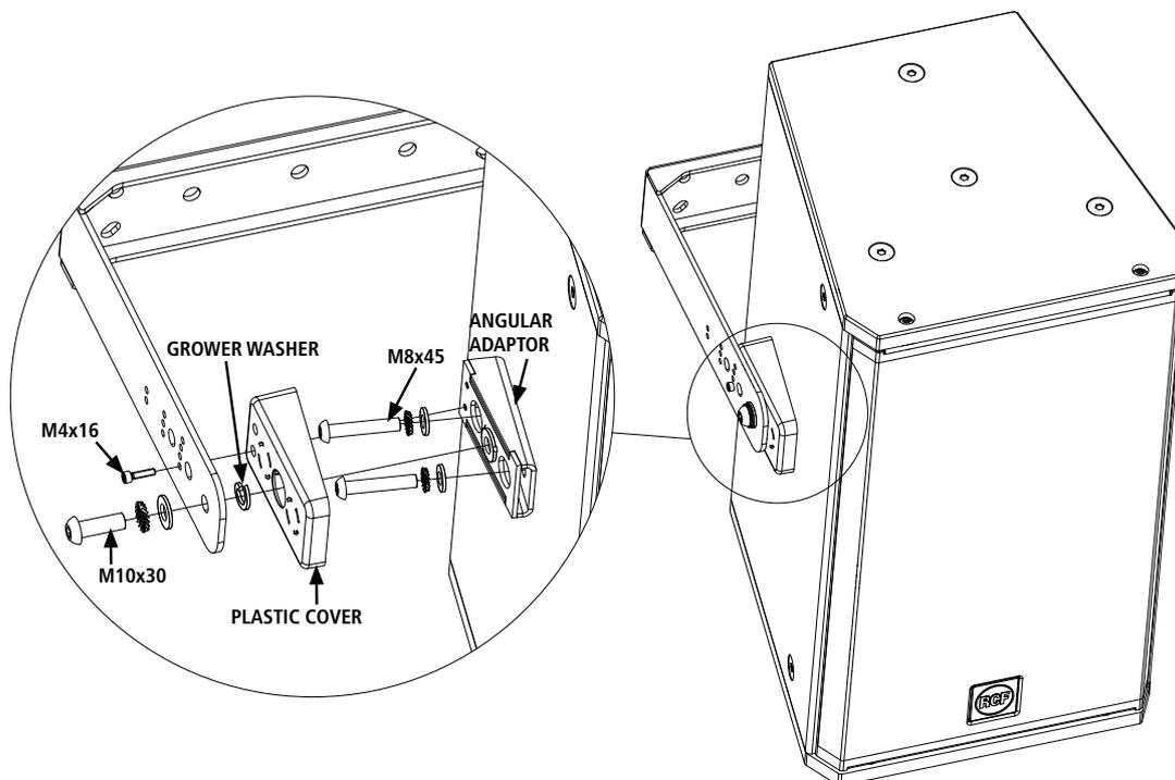
1. After removing the screws on the speaker sides, fix the angular adaptor on the speaker with the M8x45 screws.
