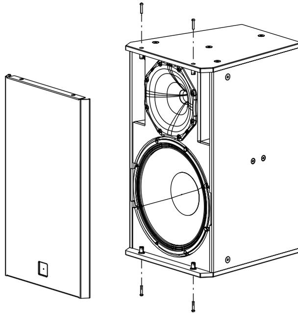
2. Remove the 8 screws from the horn and rotate it 90°
