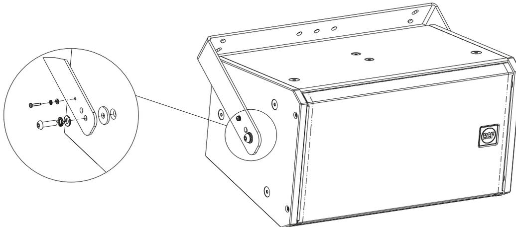
Alternatively, it's possible to install the speaker in a less protruding way by using the other two inner holes on the U bracket. Before tightening the two M10 bolts, adjust the loudspeaker vertical tilt and then (when you found the right angle) fix it through two M4.2x22 self-threading screws (passing through the small hole of the U bracket) directly into the loudspeaker cabinet wood.
