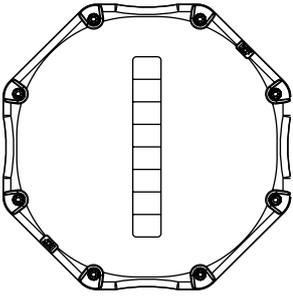
Whether the speaker is used vertically or horizontally the waveguide must always be mounted as shown on the picture on the side.
